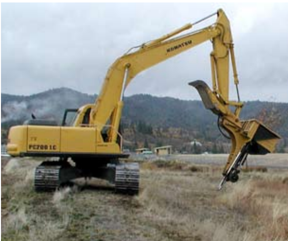
Figure 18.—The Stinger, an excavator with a boom-mounted dibble, is used to open planting holes and insert pole cuttings or large container stock. It is especially useful in rocky soils.
